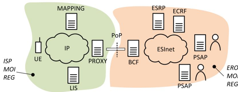
**Figure 12: ESInet terminates IP**
