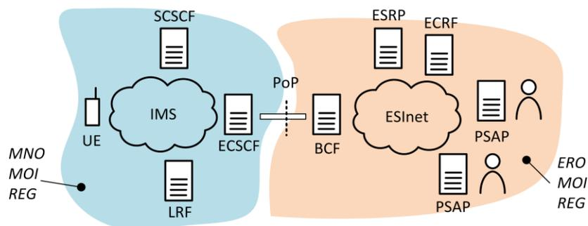
Figure 11: ESInet terminates IMS
